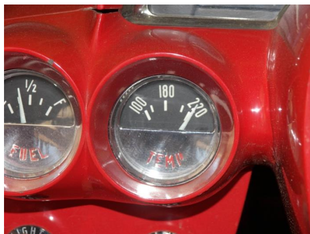
Illustration 1 – Gauge indicates overheating on an engine at normal temperature.
