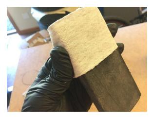
This will take some practice and several passes, and the wiping block must be held very flat. Lead with the rolled edge of fabric, not the lose edge. Move the wiping block across the grill crosswise, not lengthwise, because a crosswise movement has the ridges closer together to better support the block and keep the material from contacting the depressions. You will need to change the material often so count on sacrificing one old sweatshirt.
