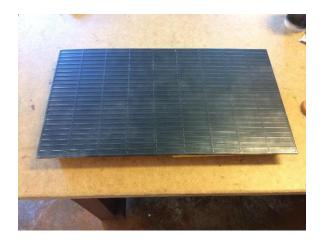
Next, take a piece of smooth fabric, like the smooth side of a cut up sweat shirt, and wrap it <u>tightly</u> around a stiff sanding block. Apply lacquer thinner to center section of the fabric, damp but not dripping, and wipe lightly over the grill to remove the paint from the ridges only.
