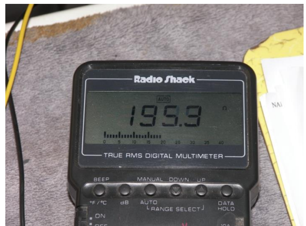
Illustration 5 - Completely normal sender resistance for an engine at ~145 degrees.
