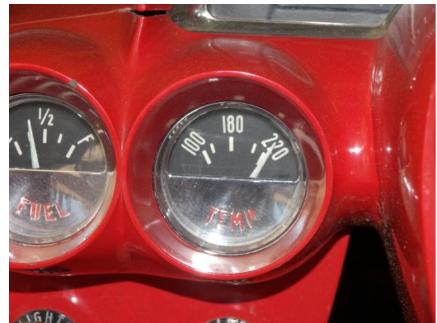
Illustration 1 – Extreme temperature indication but engine is at normal temperature.
