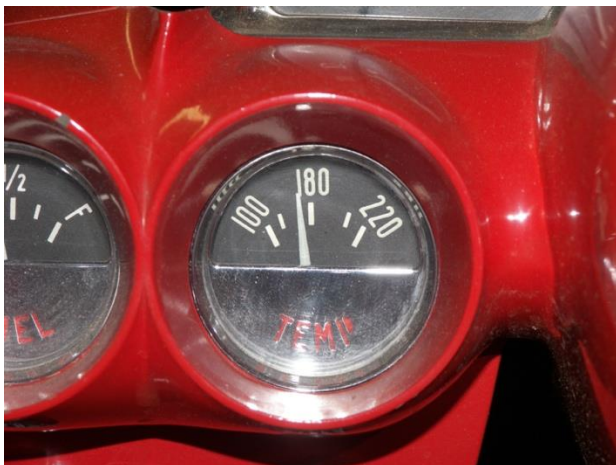
Illustration 3 - Gauge indication with fixed resistor of 128 Ohms.
