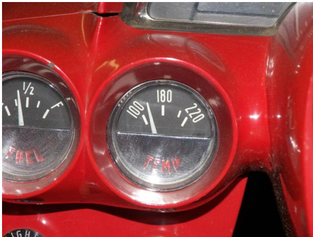
Illustration 2 - Gauge indication with fixed resistor of 147 Ohms.
