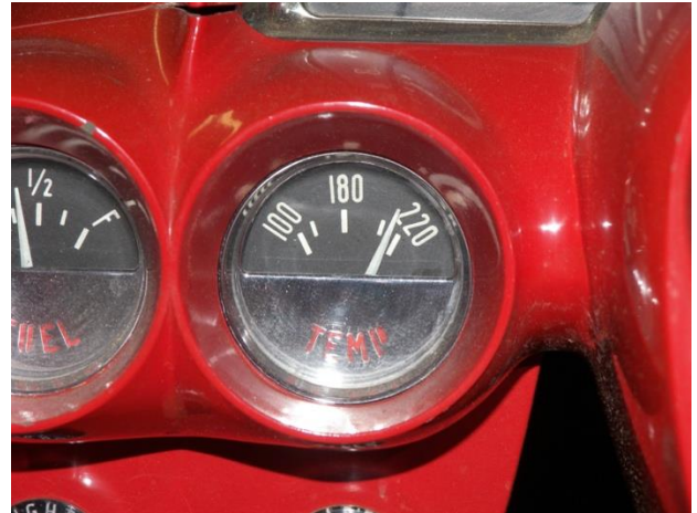
Illustration 4 - Gauge indication with fixed resistor of 104 Ohms.
