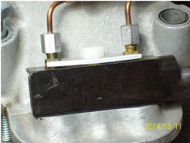
Illustration 5: Nylon bolts eliminate the conductive path between the engine and the nozzles. After a hot restart, the nozzle temperature drops measurably quicker.
