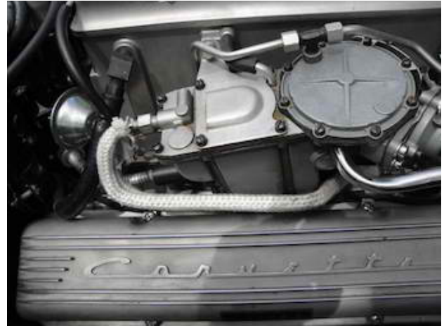
Illustration 1: Insulating fuel line reduces the heat picked up by fuel as it passes over the hot engine.
