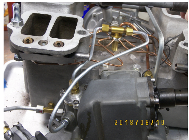
Illustration 4: The short silver tube supplies fuel to the spider. Fuel returns to the bowl via the longer silver tube. Notice the lack of insulation.
