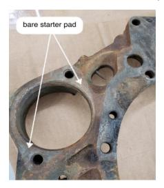
Lastly, the NEG. cable attaching point on the transmission was also cleaned to bare metal before reattaching the cable.
