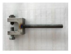
I mentioned during the August NCC meeting on Zoom that I had purchased a tool to install the two rivets that attach the grounding strap for the air cleaner base to the front of the vertical ignition shield on Sharyl's `69. Now that those two rivets are installed, the rivet tool has taken up residence in my toolbox.
