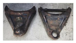
The second photo is of a 64-77 lower A-arm, that will also service 78-82. It has the original, pivot shaft, the original (not useable) bushings and the original (not useable) riveted ball joint. There is no pitting on the A-arm, just light surface rust. A-arm can be restored to like new condition with bead blasting or sanding and a new paint job or used as a core in an exchange.
