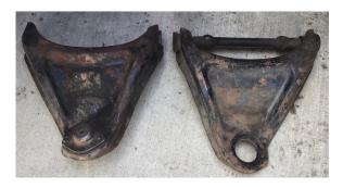
The second photo is of a 64-77 lower A-arm, that will also service 78-82. It has the original, pivot shaft, the original (not useable) bushings and the original (not useable) riveted ball joint.
