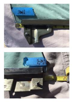
I then installed the glass and sash in the door for the third time. The first of the next two photos shows the rear access hole in the inner door surface, with the nut tightened onto the sash stud. The second of the next two photos shows the forward access hole.
