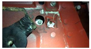
For both rear and forward holes the sash studs were well centered, and it was very easy to place and tighten the nuts with a 1/4" drive socket wrench. After securing the nuts and installing the lower rear metal window run and snapping the last bubble clip on the fuzzy channel into place, I tested the window operation. It went up and down as smooth as glass (pun intended).
