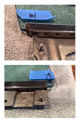
The left-hand vertical line in each pair of lines is the original location, and the right-hand vertical line is where I wanted to relocate the ends of the sash. The shift I wanted was between 3/8" and 1/2".
