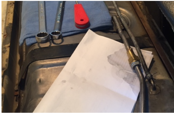
Photo #6 shows the fuel line disconnected from the sending unit assembly.
