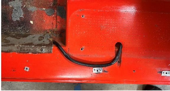
Photo 1-Initial antenna cable at sill plate.
