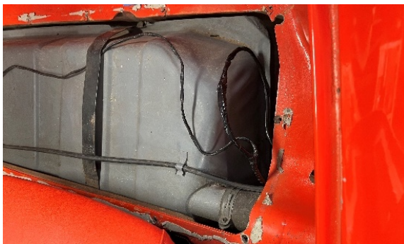
Photo 8-Final taped wires in tank area.
