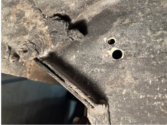
Photo 4-Drilled hole to access rocker area.
