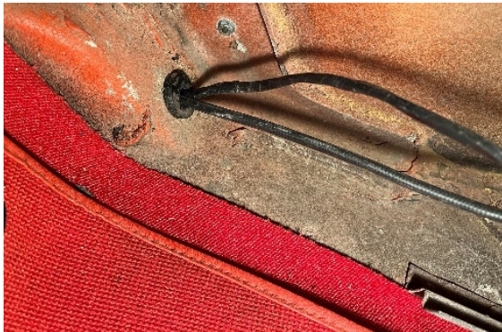
Photo 5-New wiring behind the kick panel.
