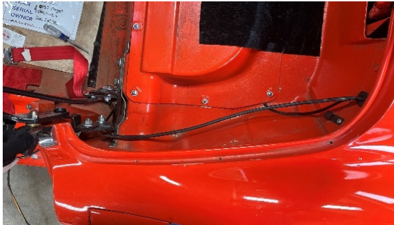
Photo 2-Initial antenna cable and trunk wiring in the soft top well.
